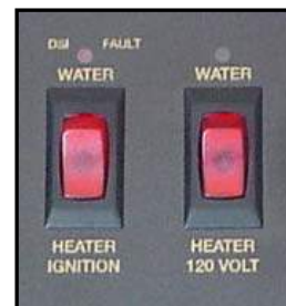
Figure 4-17. Water Heater Switches
