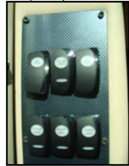
Figure 9-7. Entrance Step Switch (right middle)
