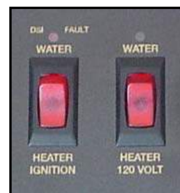
Figure 4-16. Water Heater Switches
