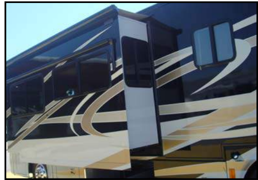
Figure 8-2. Typical Slide-Out Fully Extended
