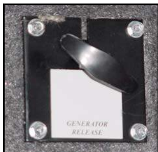
Figure 7-15. Generator "Pull" Cable Slide-Lock Release
