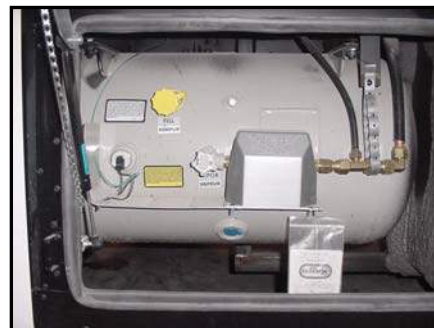
Figure 2-5. Liquid Propane Tank
