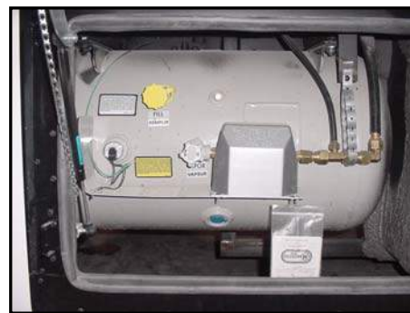
Figure 2-3. Liquid Propane Tank
