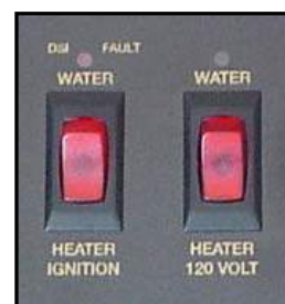
Figure 4-16. Water Heater Switches
