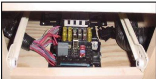
Figure 7-18. Fuse Blocks within Center Console
