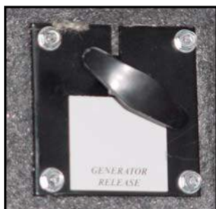
Figure 7-18. Generator “Pull” Cable Slide-Lock Release
