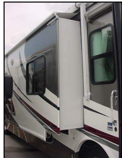
Figure 8-2. Typical Slide-Out Fully Extended
