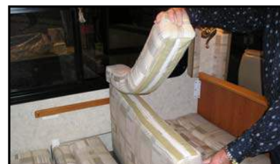
Figure 5-7. Filler Strip Attached to the Seat Portion
