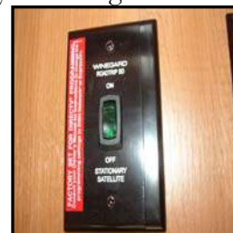
Figure 4-8. Dome Satellite Control
