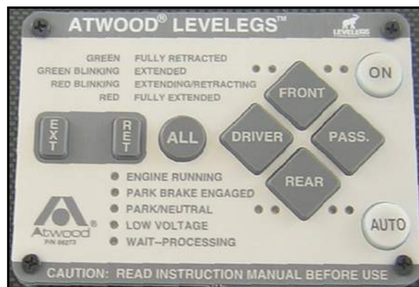
Figure 9-6. Leveling Control Panel on Dashboard
