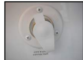
Figure 11-6. City Water Inlet
