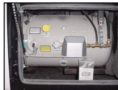
Figure 3-4. Liquid Propane Tank
