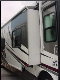
Figure 8-2. Typical Slide-Out Fully Extended
