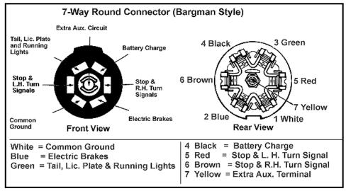
Figure 7-22. Seven-Pin Towing Connector
