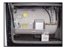
Figure 2-3. Liquid Propane Tank
