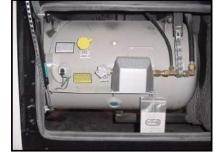
Figure 3-3. Liquid Propane Tank
