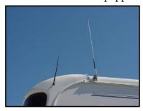
Figure 4-17. CB Radio Antenna
