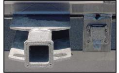
Figure 2-8. Class 3 Towing Hitch
