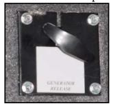
Figure 7-18. Generator "Pull" Cable Slide-Lock Release
