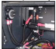
Figure 7-6. Engine Battery Disconnect Switch (left side)
