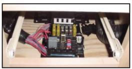
Figure 7-21. Fuse Blocks within Center Console
