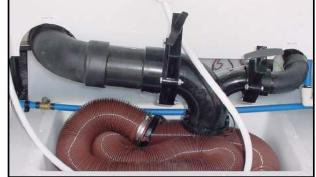
Figure 11-10. Sanitation Coupling, Valve, and Hose
