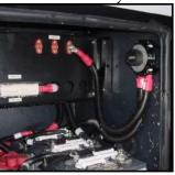
Figure 7-7. House Battery Disconnect Switch (right
