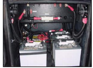
Figure 7-5. 12 VDC Battery System
