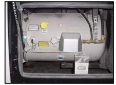
LP-appliance-lighting problems are typically caused by an improperly adjusted gas regulator. NEVER attempt to adjust or
