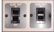
Figure 8-1. Slide-Out Switches
