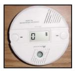
Figure 4-20. Carbon **Monoxide Detector**
