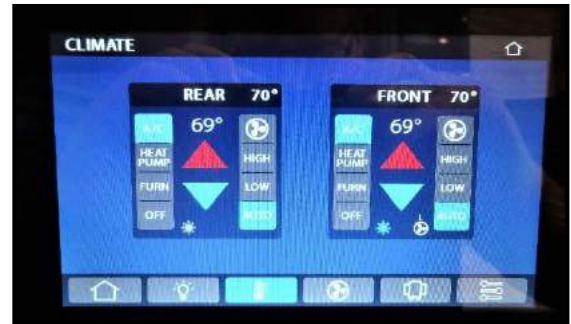
Figure 3-1: Spyder Controls System
