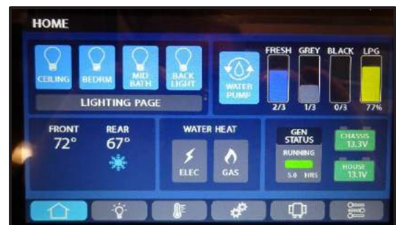
Figure 5-8: Water Heater Control Screen
