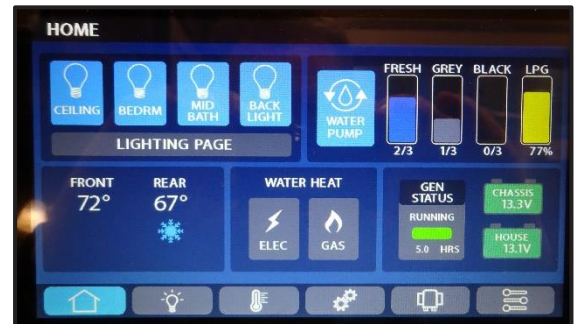
Figure 9-15: Spyder Controls Multiplexing System
