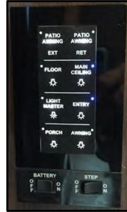
Figure 11-6: Entrance Step Switch
