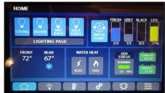
Figure 13-5: Spider Controls System Switch
