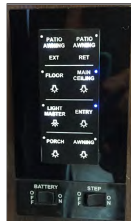
Figure 9-14: 12 VDC disconnect switch
