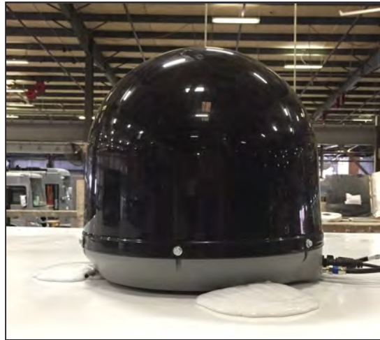
Figure 6-1: The dome satellite on top of the coach can be raised to allow easy access to change switches to a new satellite provider.
