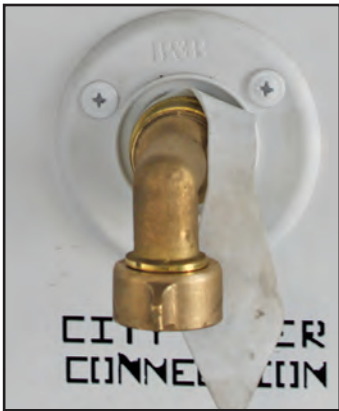
Figure 13-6: City water supply connection
