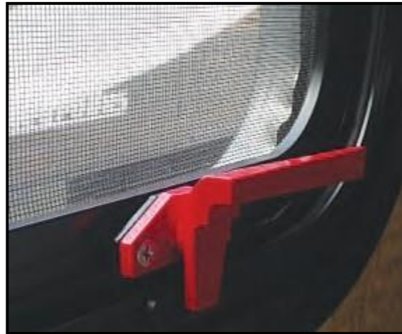
Figure 2-9: Emergency Exit Latch
