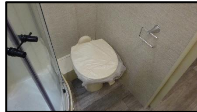
Figure 12-10: Rear Macerator Toilet
