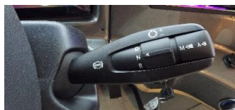
Figure 15-8 Freightliner Transmission Controls
