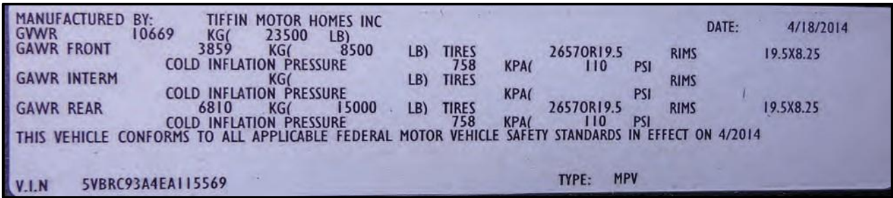
Figure 1-3: Federal Motor Vehicle Standards label located inside the doorway of the coach
