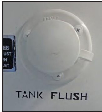
Figure 13-12: Tank Flush Connection
