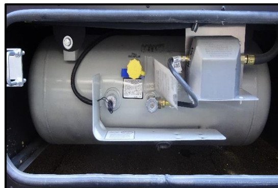
Figure 2-2: LP Tank and Regulator
