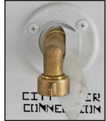
Figure 13-7: City Water Supply Connection
