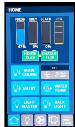
Figure 9-1: Spyder Controls System
