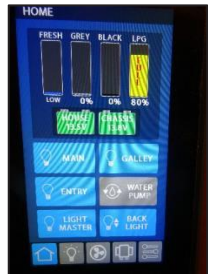
Figure 13-5: Spider Controls System Switch
