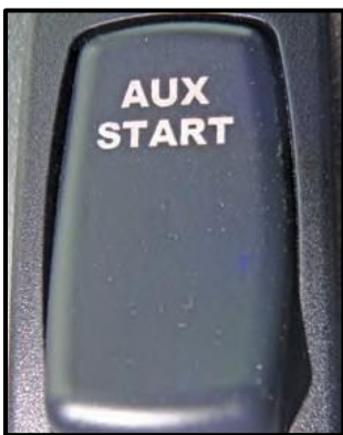
Figure 9-18: Auxiliary Start Switch
