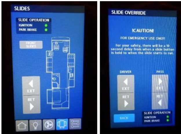
Figure 10-1: Slide-Out Screen on the Spyder Controls System
