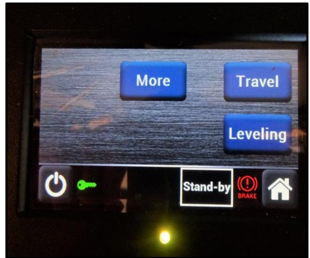
Figure 15-5: Leveling System Control Panel
