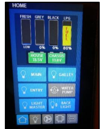
Figure 9-1: Spyder Controls System
