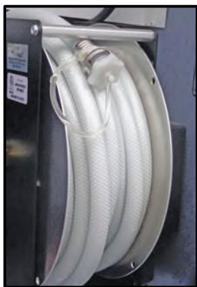
Figure 13-6: Motorhome Water Hose
