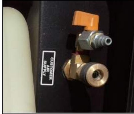
Figure 8-2: Rear Customer Air Supply
