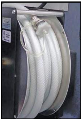
Figure 13-6: Motorhome Water Hose
