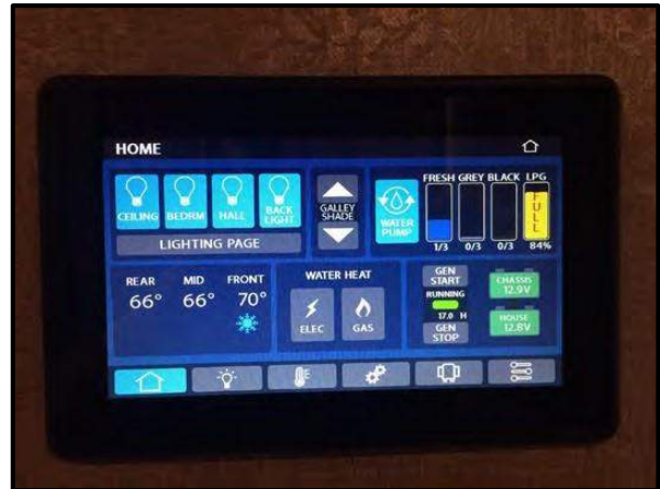
Figure 9-1: Spyder Controls System
