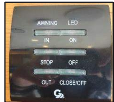
Figure 14-3: Patio Awning Control Switch
