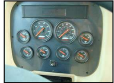
Figure 14-16. Dashboard and Instrumentation Panel
