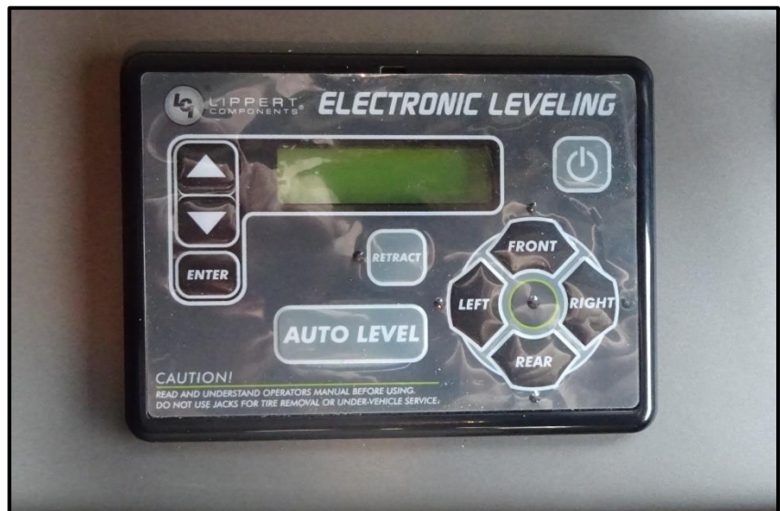
Figure 15-5: Leveling System Control Panel
