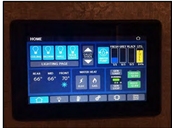
Figure 9-1: Spyder Controls System
