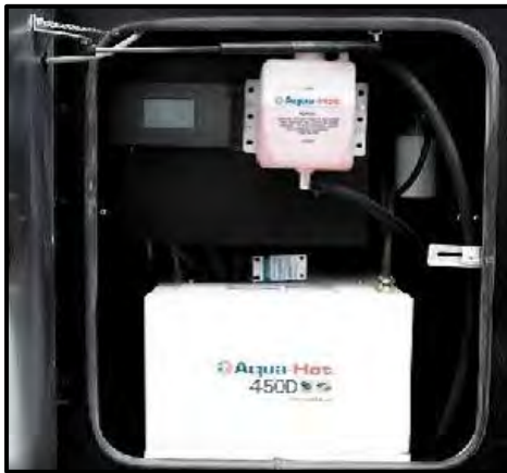
Figure 3-7: Aqua-Hot Surge Tank
