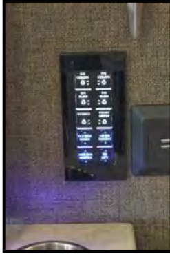
Figure 6-6: Television Lift Control Panel (located in the living room slide-out box)
