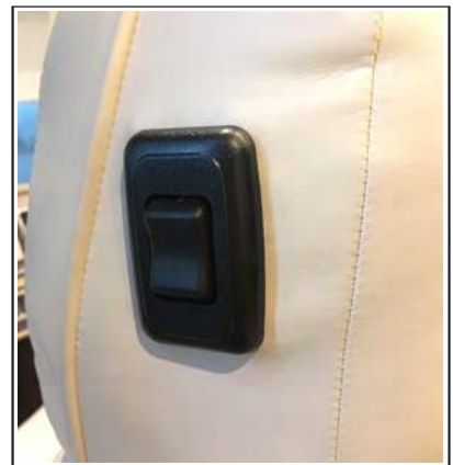
Figure 10-1b: Slideout Switch on Driver's / Passenger's Seat
