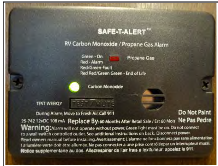
Figure 2-6: LP Gas Detector
