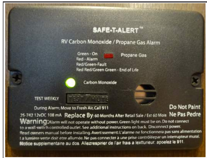
Figure 2-6 : LP Gas Detector
