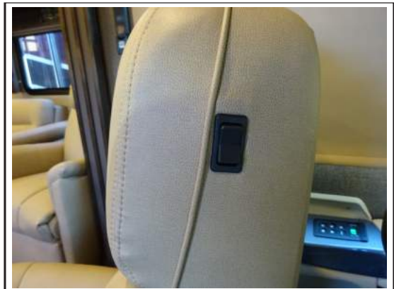
Figure 10-1b: Slideout Switch on Driver's / Passenger's Seat
