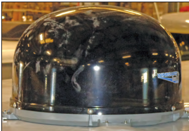
Figure 6-1: The dome satellite on top of the motorhome can be raised allowing easy access to change dip switches to a new satellite provider.
