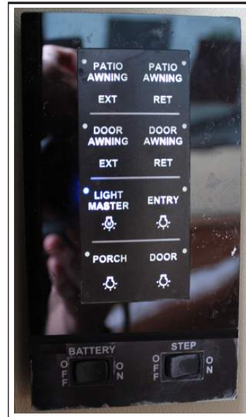
Figure 9-13: 12 VDC disconnect switch
