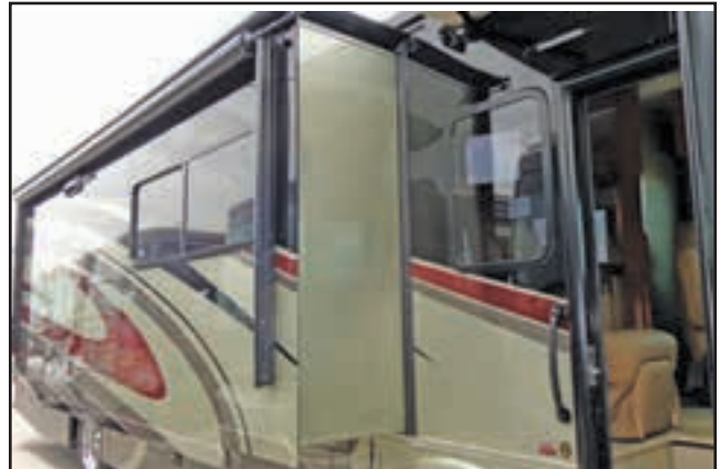
Figure 10-2: Typical slide-out fully extended
