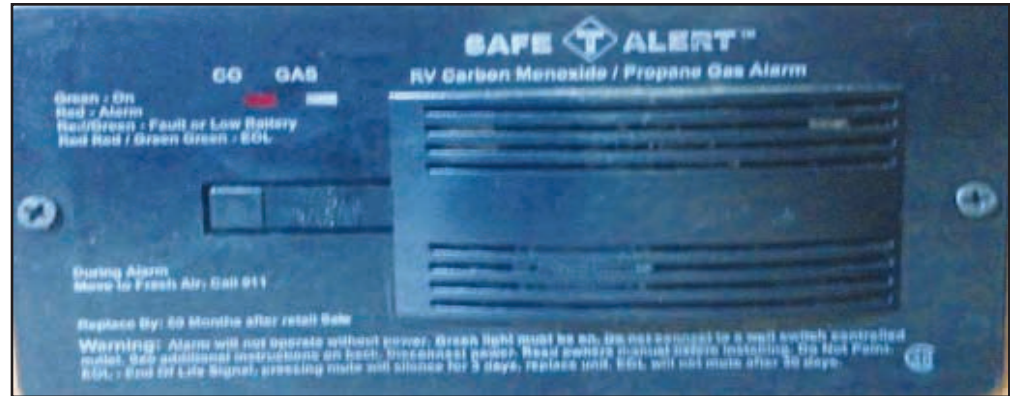
Figure 2-6: Carbon Monoxide alarm
