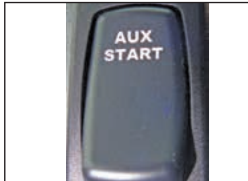
Figure 9-13: Auxiliary start switch
