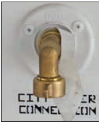
Figure 13-6: City water supply connection
