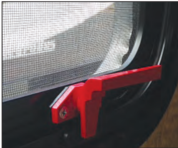
Figure 2-10: Emergency exit latch
