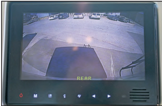
Figure 15-1: Rear-view camera monitor system
