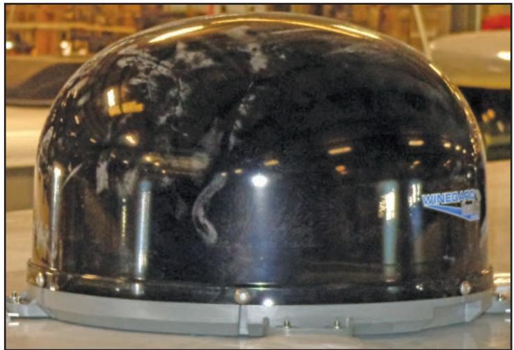
Figure 6-1: The dome satellite on top of the motorhome can be raised allowing easy access to change switches to a new satellite provider.
