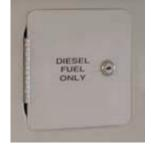
Figure 2-4. Gas Tank Port
