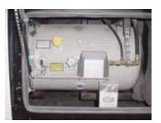
Figure 2-3. Liquid Propane Tank
