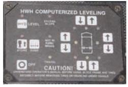
Figure 9-5. HWH Computerized Leveling System
