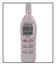
Figure 13-4. Portable Hygrometer
