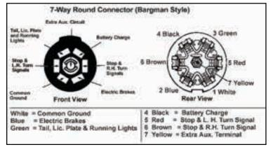
Figure 7-16. Seven-Pin Towing Connector
