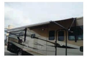
Figure 12-3. Power Patio Awning (Fully Extended)
