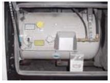
Figure 2-5. Liquid Propane Tank
