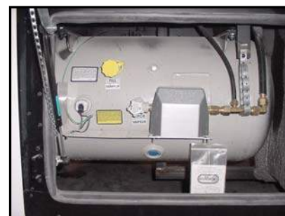
Figure 3-4. Liquid Propane Tank
