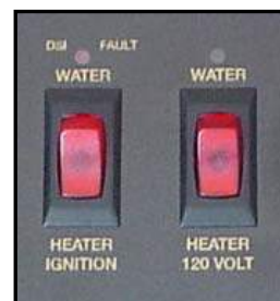
Figure 4-16. Water Heater Switches
