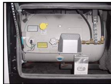
Figure 2-5. Liquid Propane Tank
