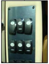
Figure 7-8. 12 VDC Disconnect Switch
