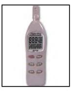
Figure 14-5. Portable Hygrometer
