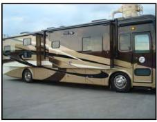
Figure 8-2. Typical Slide-Out Fully Extended
