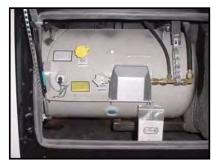
Figure 3-4. Liquid Propane Tank
