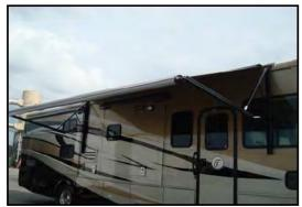
Figure 12-3. Power Patio Awning (Fully Extended)
