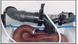
Figure 11-11. Sanitation Coupling, Valve, and Hose
