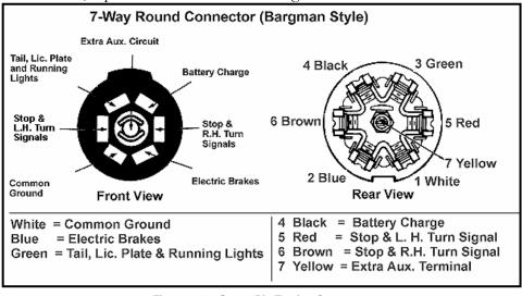
Figure 7-16. Seven-Pin Towing Connector
