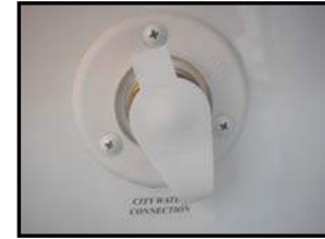
Figure 11-6. City Water Inlet
