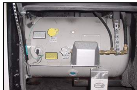
Figure 2-3. Liquid Propane Tank
