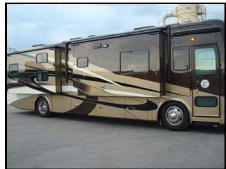
Figure 8-2. Typical Slide-Out Fully Extended
