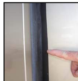
Figure 14-6. Inspecting Slide Out Gasket
