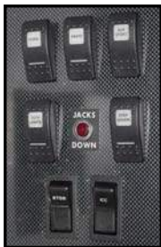
Figure 7-3. Auxiliary Start Switch
