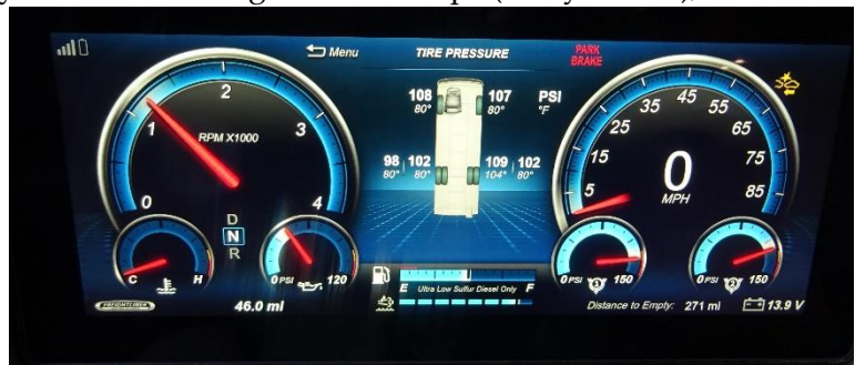
Figure 16:4 Instrument Panel Tire Pressure Monitor
