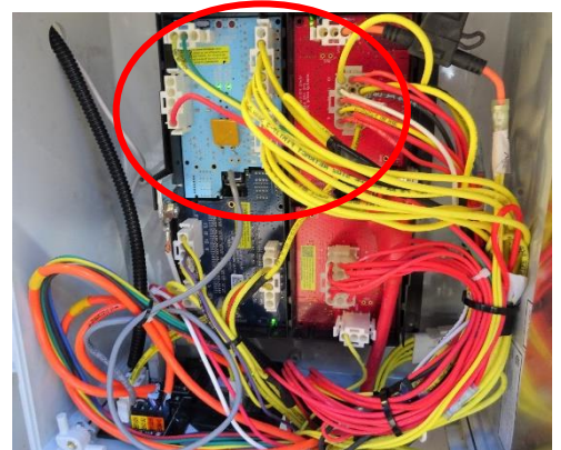
Figure 10-4: Location of Slide-Out Room Control Override
