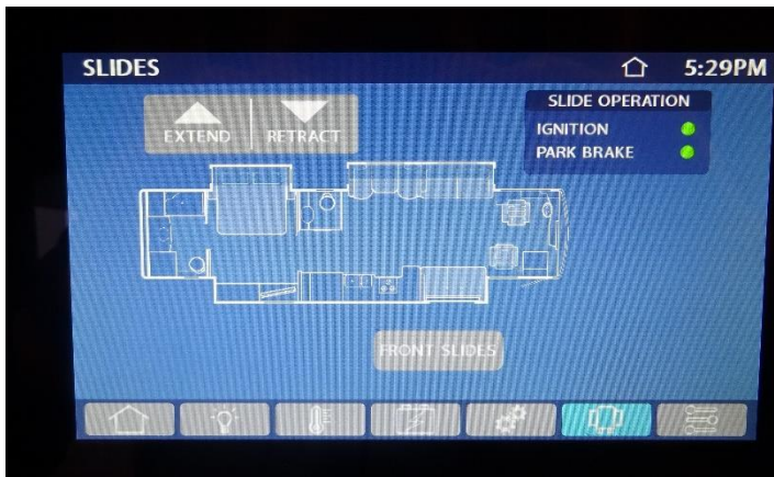
Figure 10-1: Slide-Out Screen on the Spyder Controls System
