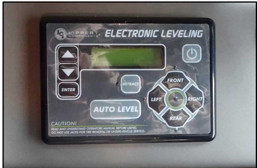
Figure 15-5: Leveling System Control Panel
