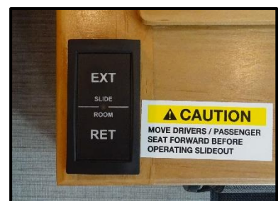
Figure 10-2: Front Slide-Out Switch
