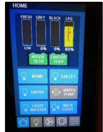
Figure 9-1: Spyder Controls System
