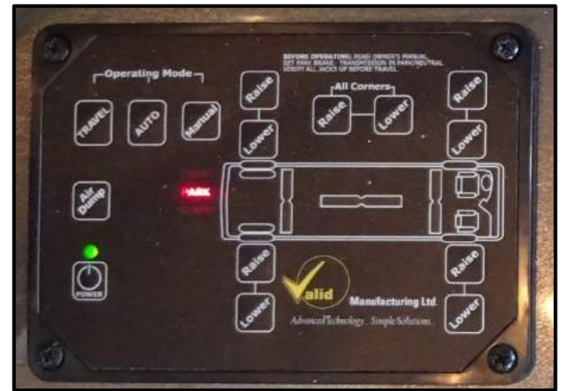
Figure 15-10: Levelling System Control
