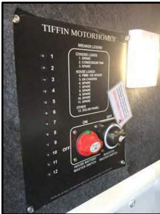
Figure 9-15: House Battery Disconnect Panel
