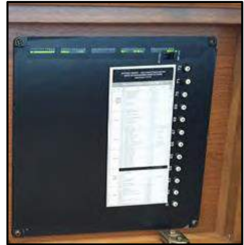
Figure 9-3: Multiplex System Switch Panel
