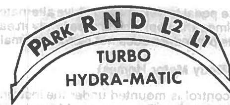
Turbo Hydra-Matic Shift Positions TRANSMISSION SELECTOR LEVER (A Body Motor Homes)
