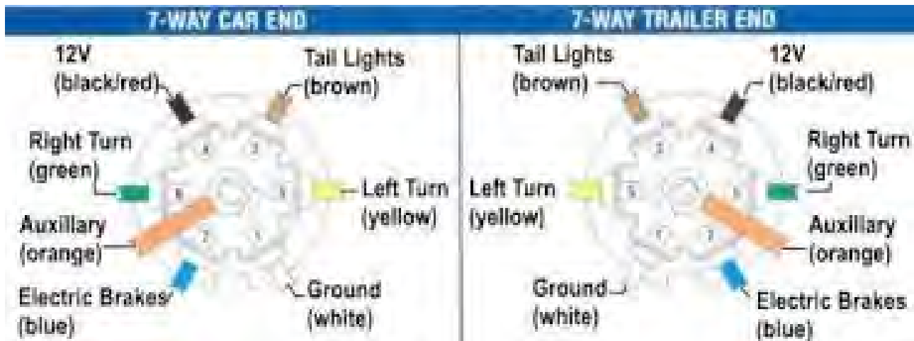
Figure 9-13: Seven Pin Connector Diagram
