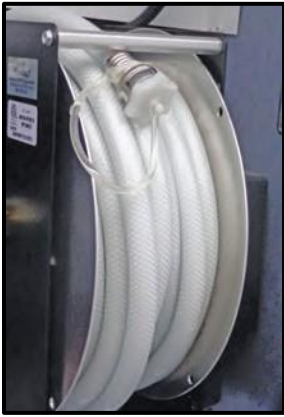
Figure 13-6: Motorhome Water Hose
