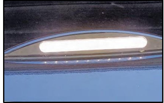
Figure 11-3: Exterior Security Light
