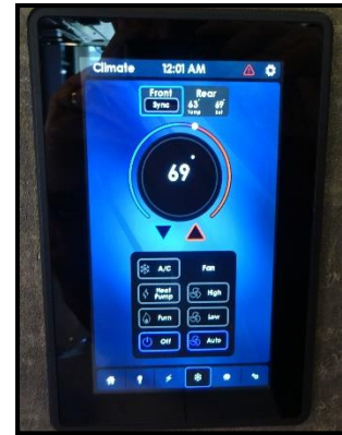
Figure 3-1: Spyder Controls System
