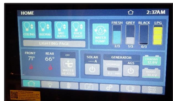
Figure 13-5: Spider Controls System Switch
