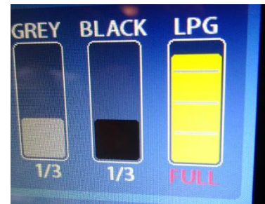
SPYDER Control showing approximate amount of LP Gas Remaining in Tank.
