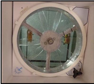
Figure 14-3: Overhead Vent Fan
