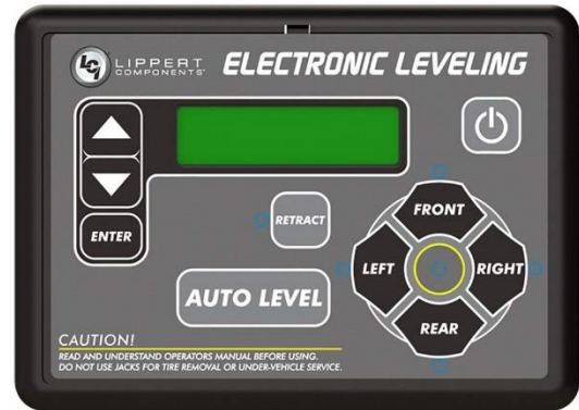
Figure 15-5a: Lippert Control Panel
