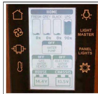
Figure 13-5: Water pump switch
