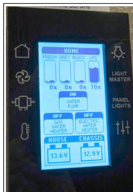
Figure 5-7: Water heater screen Spyder control system
