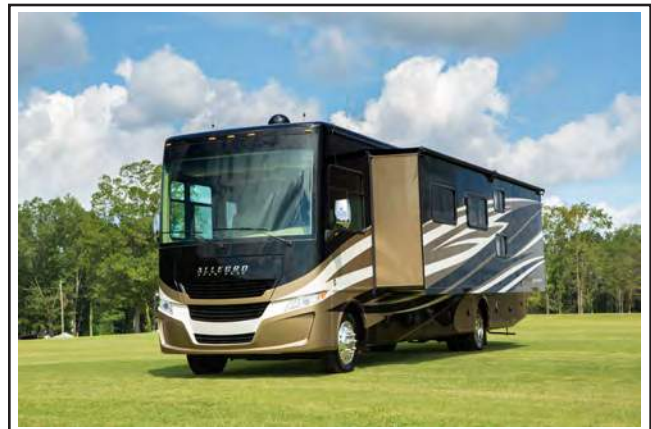
Figure 10-2: Typical slide-out fully extended
