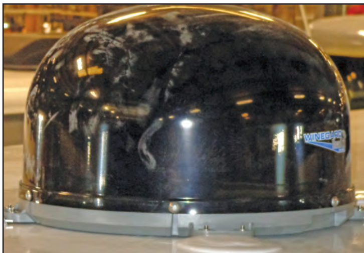
Figure 6-1: The dome satellite on top of the motorhome can be raised allowing easy access to change switches to a new satellite provider.
