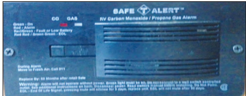
Figure 2-6: Carbon Monoxide alarm
