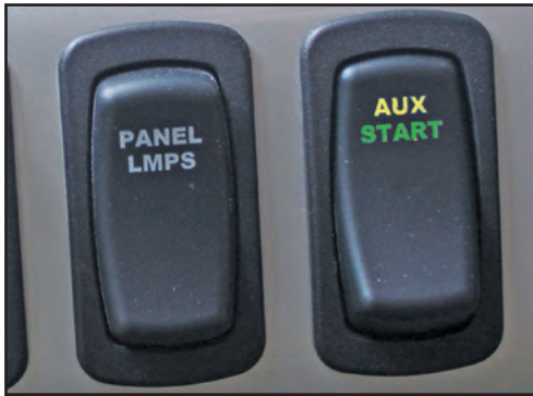
Figure 9-2: Auxiliary start switch
