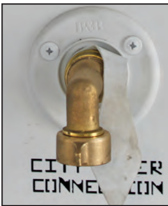
Figure 13-6: City water supply connection
