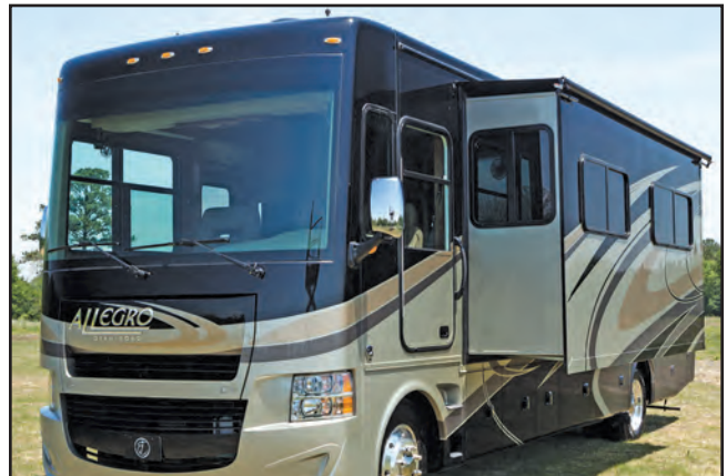
Figure 10-2: Typical slide-out fully extended
