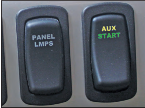
Figure 9-2: Auxiliary start switch
