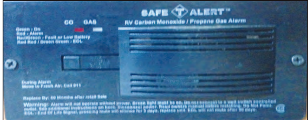
Figure 2-6: Carbon Monoxide alarm
