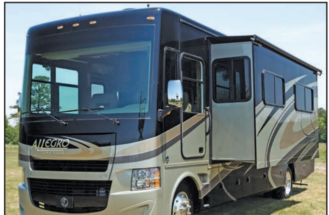
Figure 10-2: Typical slide-out fully extended
