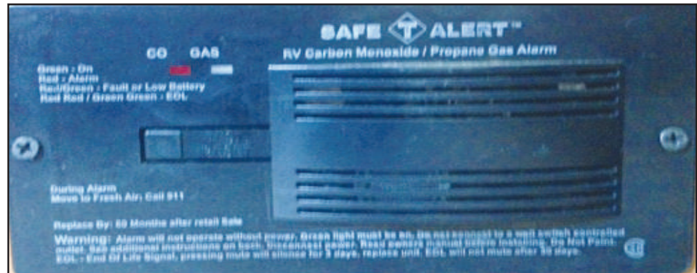
Figure 2-6: Carbon Monoxide alarm
