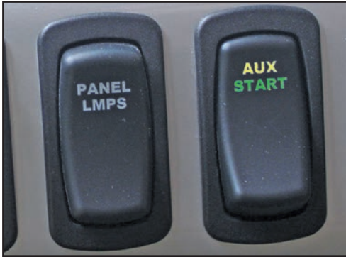
Figure 9-2: Auxiliary start switch
