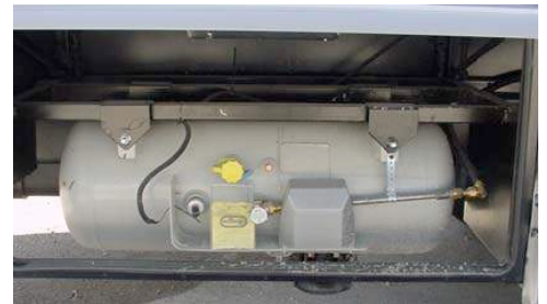
Figure 2-2. Liquid Propane Tank
