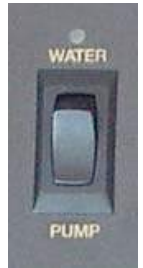
Figure 11-5. Water Pump Switch
