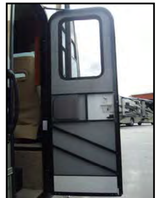
Figure 12-6. Front Door & Screen Door
