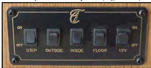
Figure 7-4. Battery Disconnect Panel
