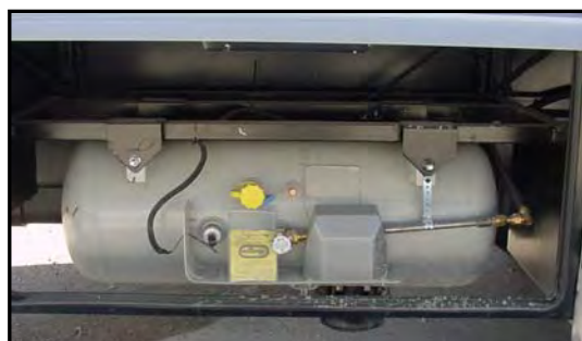
Figure 2-2. Liquid Propane Tank
