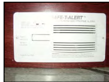
Figure 3-6. CO/LP Gas Detector
