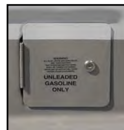
Figure 2-3. Fuel Tank Fill Door
