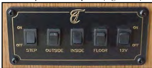
Figure 7-4. Battery Disconnect Panel
