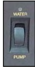
Figure 11-5. Water Pump Switch
