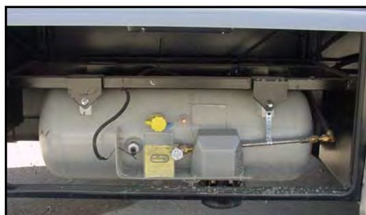
Figure 2-2. Liquid Propane Tank
