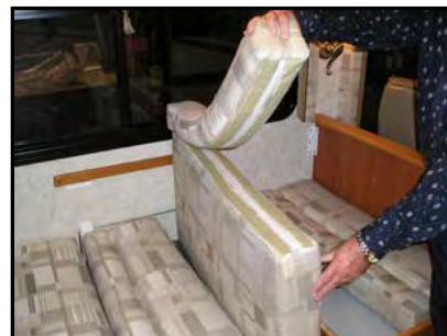
Figure 5-7. Filler Strip Attached to the Seat Portion
