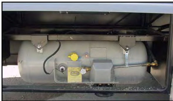
Figure 2-4. Liquid Propane Tank
