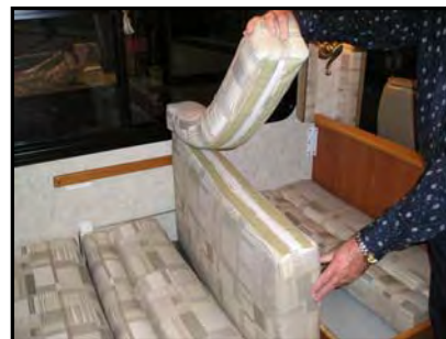
Figure 5-7. Filler Strip Attached to the Seat Portion
