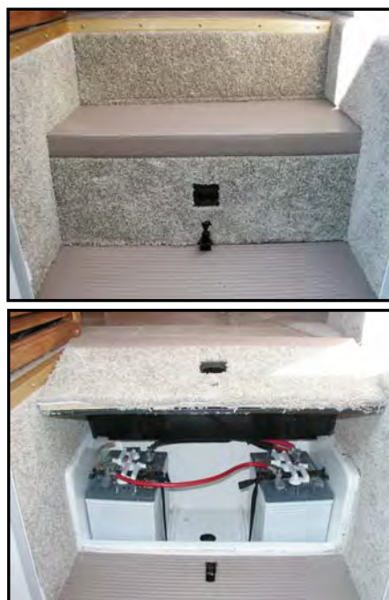
Figure 7-3. Stairwell (Top) and Battery Storage Underneath (Bottom)
