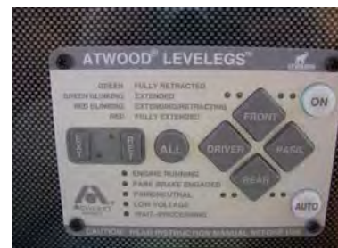
Figure 9-5. Leveling Control Panel on Dashboard
