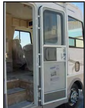
Figure 13-6. Front Door & Screen Door
