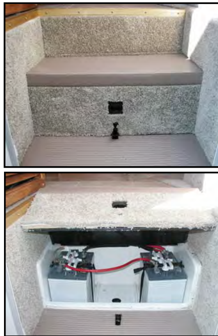
Figure 7-3. Stairwell (Top) and Battery Storage Underneath (Bottom)
