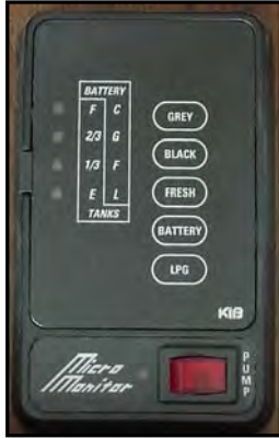
Figure 11-1. Monitor Panel (Water, LP Gas, Battery)
