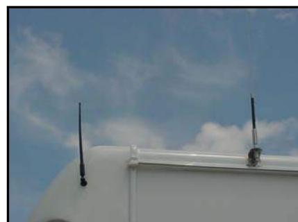
Figure 4-14. CB Antenna Installation
