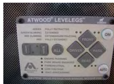
Figure 9-5. Leveling Control Panel on Dashboard
