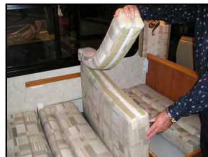
Figure 5-7. Filler Strip Attached to the Seat Portion
