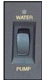
Figure 11-5. Water Pump Switch
