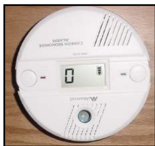
Figure 4-16. Carbon Monoxide Detector
