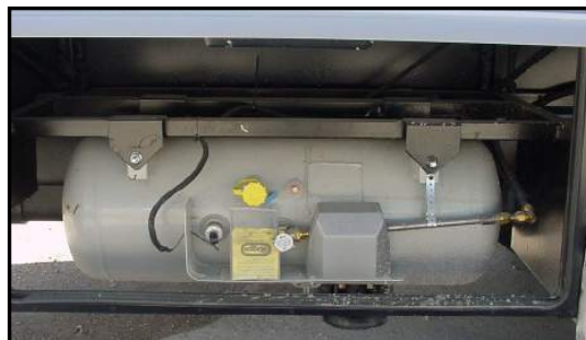
Figure 2-2. Liquid Propane Tank
