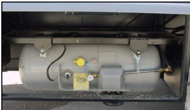
Figure 3-3. Liquid Propane Tank
