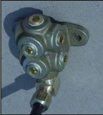
Figure 8-1: Front Customer Air Supply
