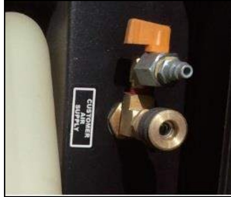
Figure 8-2: Rear Customer Air Supply
