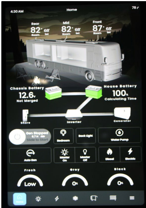
Figure 3-1: Spyder Controls Multiplex System -Home Screen Display
