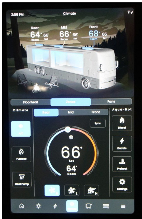
Figure 13-19: Aqua-Hot Heating System Control Screen
