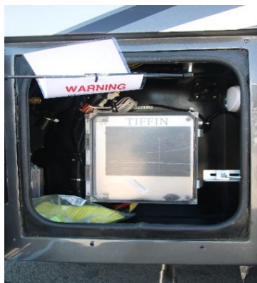
Figure 10-4: M1 Spyder Enclosure located in the driver's side exterior compartment.
